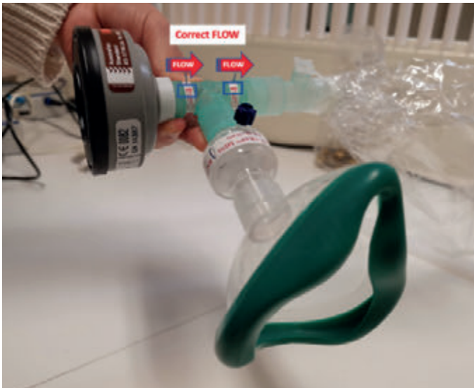
Figure 1: Example of the portable breath sampling setup used for breath collection. Credits to the breath research group of the Amsterdam UMC.
